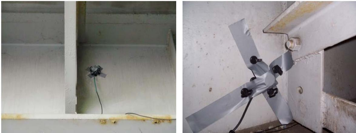
Figure 7: Typical views of AE sensors attached to the girder.
